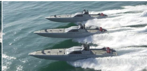
Twin V12 Seateks, Quad Turbocharged Diesels paired with Jets/Surface Drives are Top choice for Racing/Military Applications. Its Lamborgxxxii at sea, well even they are using it.
